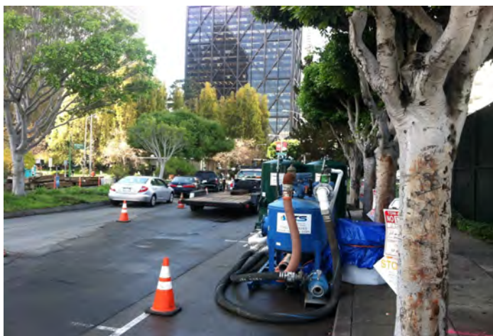
100 GPM Groundwater Treatment System in San Francisco
